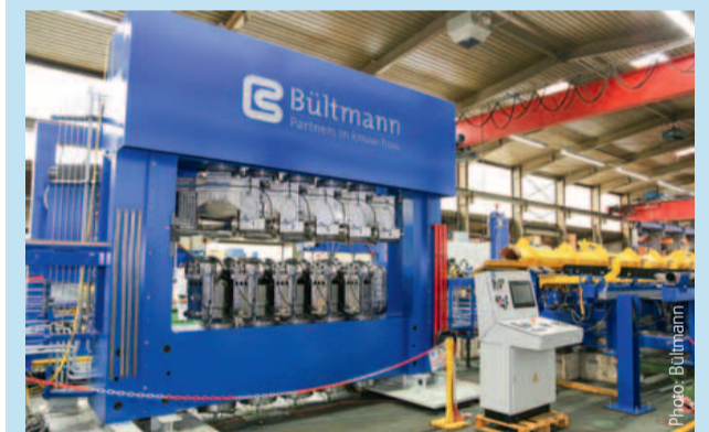
Today for straightening of precision tubes mainly 10-roll straightening machines are used
