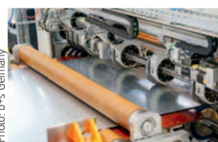
Fully automatic slitting shear with high precision
